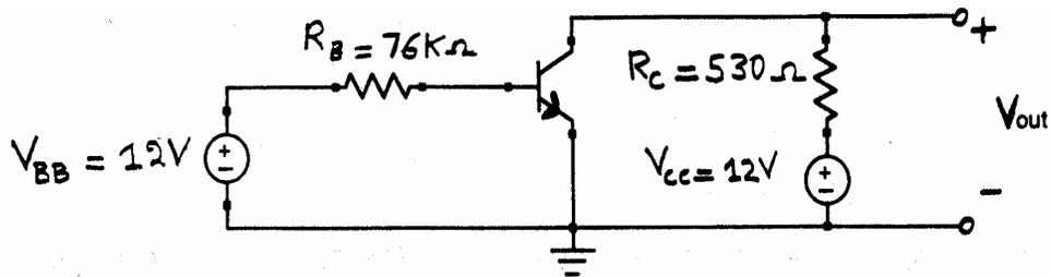
(c) Assuming  $V_{BE} = 0.6V$  and a Forward Active BJT, find the numerical value of  $V_{out}$  (in Volt).
