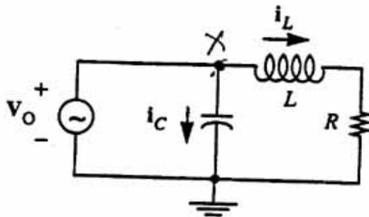
In the above circuit,  $V_0 = 10$  V (real,  $C = 10^{-8}$  F,  $L = 2 \times 10^{-4}$  H,  $R = 100$  ohms,  $\omega = 10^6$  radians/sec.
