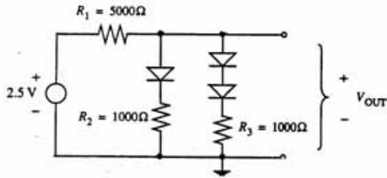
Find  $V_{out}$  in the above circuit. The diodes are to be represented by the large-signal diode model (including the 0.7 V drop across a forward-biased diode.) **Make sure your answer is reasonable and consistent.** Explain your reasoning.
