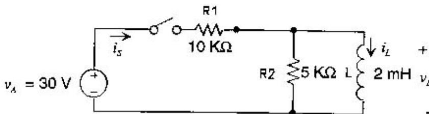
The switch has been closed for a long time, and at  $t = 0$ , the switch is opened.
