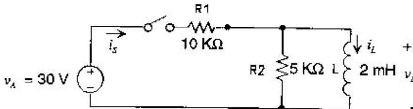
The switch has been closed for a long time, and at  $t = 0$ , the switch is opened.
