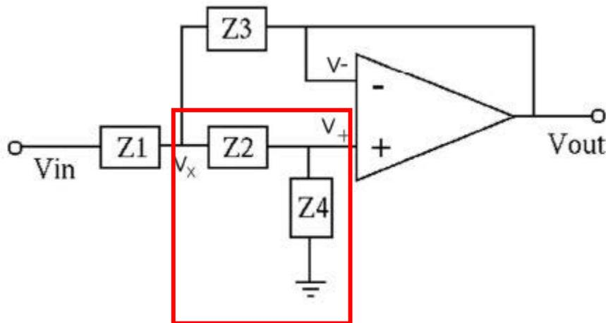
from the negative feedback, we know  $V_+ = V_- = V_{out}$
