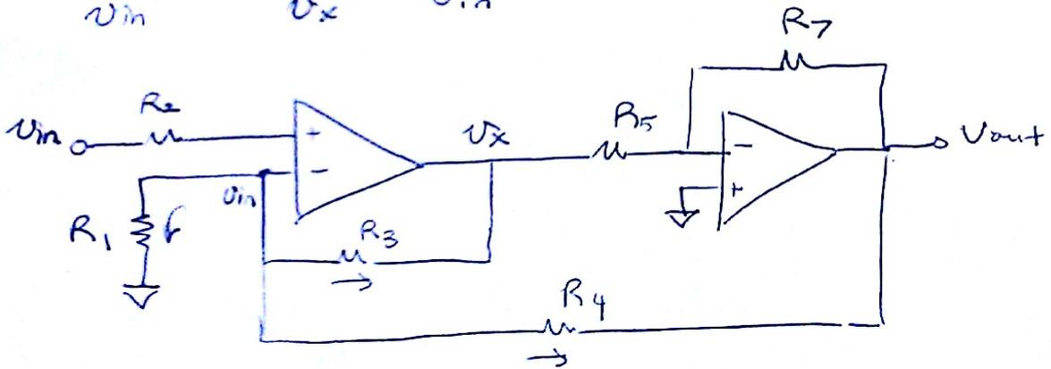
$$\frac{V_{in}}{R_1} + \frac{V_{in} - V_x}{R_3} + \frac{V_{in} - V_{out}}{R_4} = 0$$
