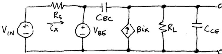
$$i_x = \frac{V_{IN} - V_{BE}}{R_S}$$
