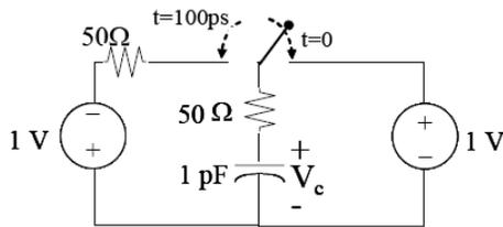
(a) At  $t < 0$ , the switch is open and  $V_c = 0$ . At  $t = 0$ , the switch is closed towards the right.
