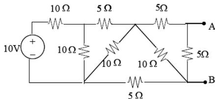
(a) What is equivalent resistance  $R_{eq}$  for points A-B?
