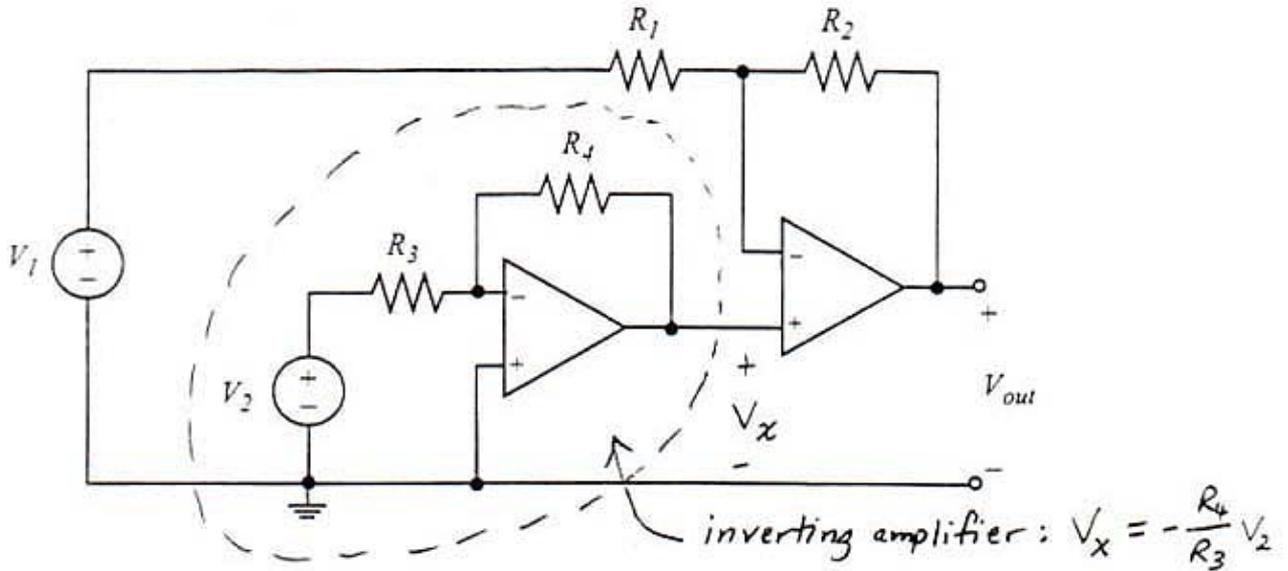
Find  $V_{out}$  in terms of  $V_1$ ,  $V_2$ ,  $R_1$ ,  $R_2$ ,  $R_3$ ,  $R_4$  [10 pts] (Hint: The superposition method might be helpful here.)
