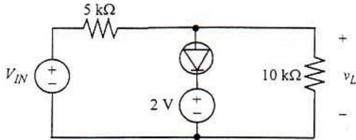
When the diode is off, we have a simple voltage-divider circuit
