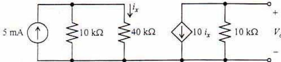
Current divider formula:  $i_x = (10 \text{ kohm}/(10 \text{ kohm} + 40 \text{ kohm})) * 5 \text{ mA} = 1 \text{ mA}$
