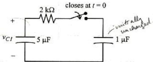
c) The following is a circuit model for an NMOS inverter, in which the transistor is turned on at time  $t = 0$ :
