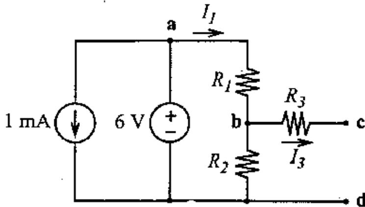
$$\begin{aligned} R_1 &= 1 \text{ k}\Omega \\ R_2 &= 2 \text{ k}\Omega \\ R_3 &= 2 \text{ k}\Omega \end{aligned}$$
