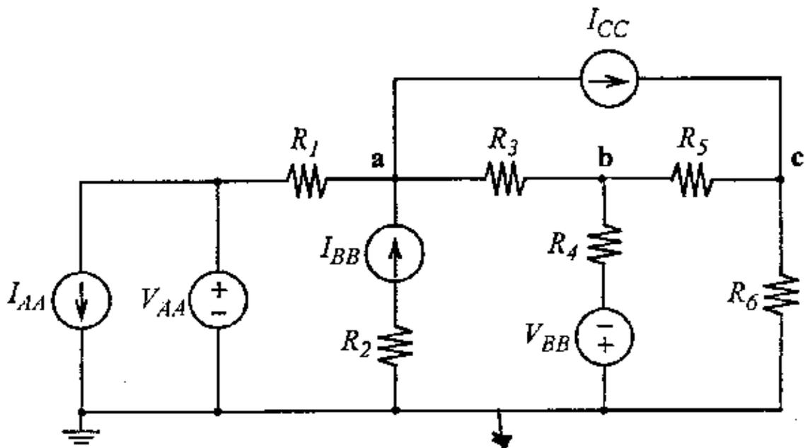
b) Similarly to part (a), use the nodal analysis technique to write 3 equations sufficient to solve for  $V_a$ ,  $V_b$ , and  $V_c$ . [10 points]
