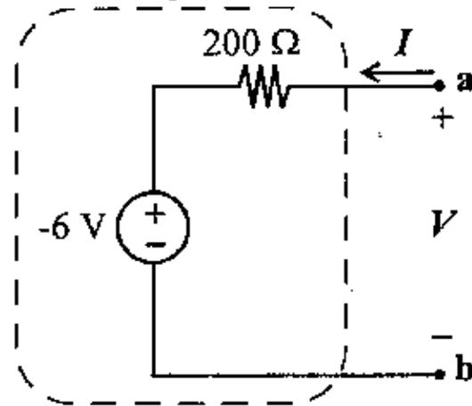
d) The circuit in part (c) is connected to a  $1\text{ k}\Omega$  load resistor (placed between the terminals **a** and **b**). Find the power absorbed in the load resistor,  $P_{1k}$  (this is what it says on the test, don't ask me). [5 points]
