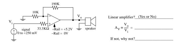
(b) You also find the following circuit. Again you suspect a linear amplifier. You know the differential amplifier has very high internal gain.
