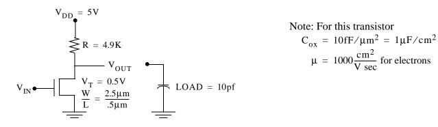
(a) If  $V_{IN} = 5V$ , what is the channel electron charge (coulomb/cm<sup>2</sup>)(for small values of  $V_{OUT}$  only)?
