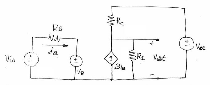
c) What is the Thevenin voltage of the Thevenin equivalent of this circuit when seen across the  $V_{out}$  terminals? (5 points)
