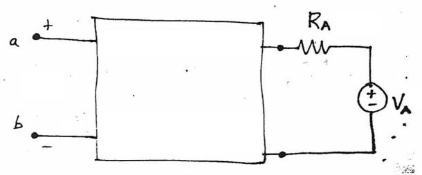
The open circuit voltage across terminals a,b is 5V. The short circuit current from terminal a to b is 2.5 A.
