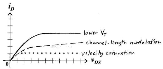
Indicate how this characteristic would change (by drawing the modified  $i_D$ - $v_{DS}$  characteristic with appropriate changes in  $I_{DSAT}$  and  $V_{DSAT}$ ):
