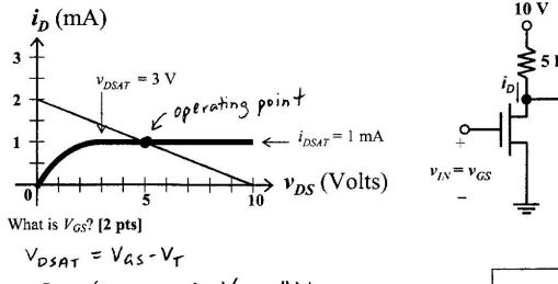
$$V_{DSAT} = V_{AS} - V_{T}$$
