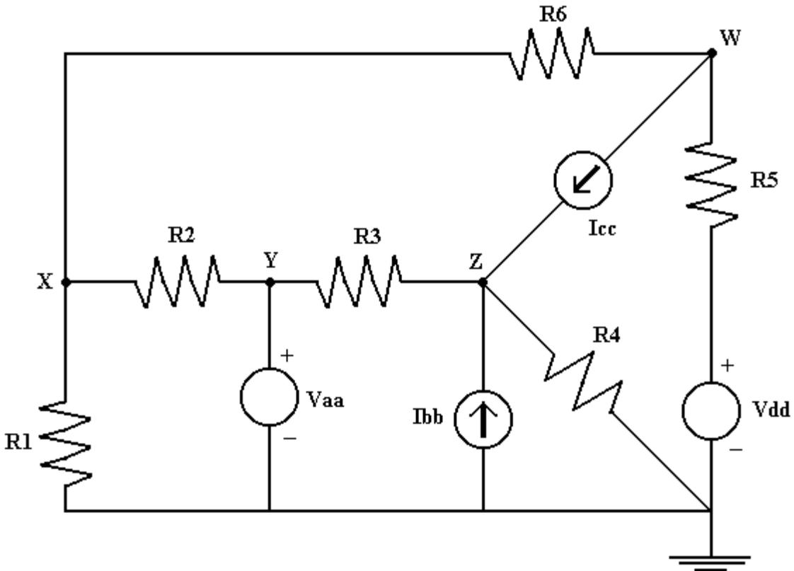
(a) In this problem you are to use nodal analysis to find a set of equations enabling you to find the values of  $V_X$ ,  $V_Y$ ,  $V_Z$ , and  $V_W$ . First, identify which of the four are really unknown node voltages and secondly, write sufficient equations to find the four values. Hint: If, for example, two of the voltages are known, you first write these two values (known node voltages), then you would need two nodal equations for the two unknowns.
