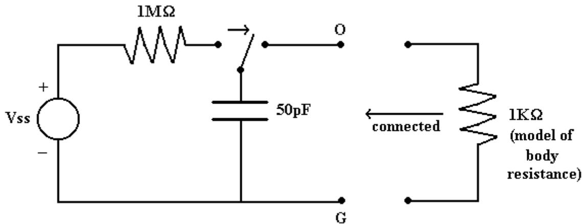
(b.1) Suppose Charlie has a response at a voltage of  $V_{SS} = 1\text{KV}$ . How much energy are you delivering to him in one pulse under such conditions?
