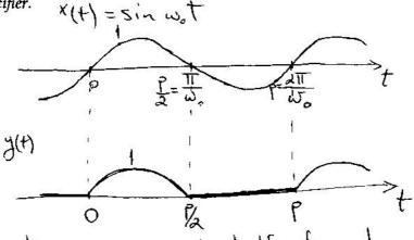
The system passes only half of each wave cycle and zeroes out the other half -> It is called a half-wave rectifier.
