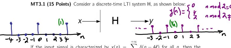
If the input signal is characterized by  $x(n) = \sum_{\ell=-\infty}^{+\infty} \delta(n-4\ell)$  for all n, then the corresponding output signal is
