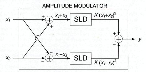
Each square-law device is characterized by the following parabolic input-output graph, where  $x_{\mathsf{SLD}}$  denotes the input to the SLD and  $y_{\mathsf{SLD}}$  the output. The parameter K is a positive constant.
