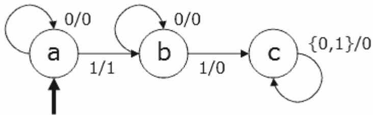
Draw the diagram of a two-state machine, Machine B, that simulates Machine A. Give the simulation relation.
