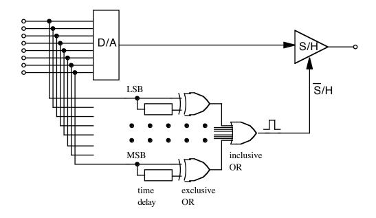
**4.3** When any input bit changes, the time delay will cause the exclusive OR to change state. The pulse produced has a width equal to the time delay. The output of the inclusive OR will be high whenever any bit changes. This puts S/H into hold mode during the glitch and the glitch will not appear at the output.
