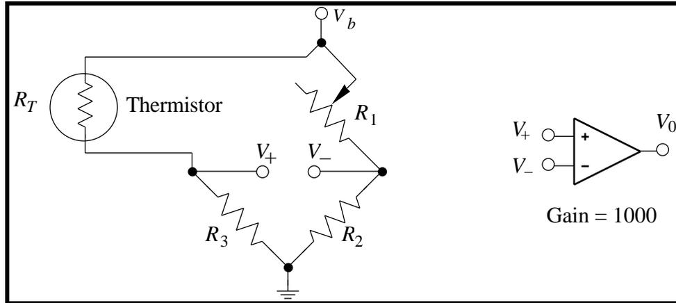
**3b**  $\text{Gain} = V_0 / (V_+ - V_-) = (1 \text{ V}) / (0.00100 \text{ V}) = 1000$ ,  $\text{Bandwidth} = 10^6 \text{ Hz} / 1000 = 1000 \text{ Hz}$ .
