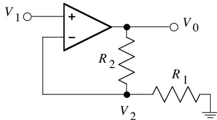
The op-amp has open loop gain  $A = k/f$ ,  $k = 10^6$  Hz and the input impedances are infinite.
