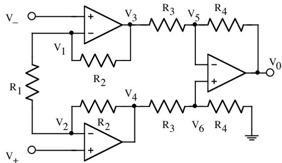
2.1 (10 points) Derive an equation for the **common mode gain**  $(V_4+V_3)/(V_++V_-)$  of the **first stage** of the above instrumentation amplifier. Assume the virtual short rule for all op-amps.
