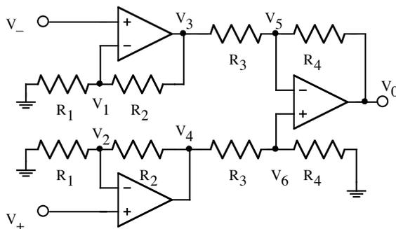
**3.1** (10 points) Derive an equation for the **common mode** gain  $(V_4+V_3)/(V_++V_-)$  of the **first stage** of the new instrumentation amplifier design shown above. Assume the virtual short rule for all op-amps.
