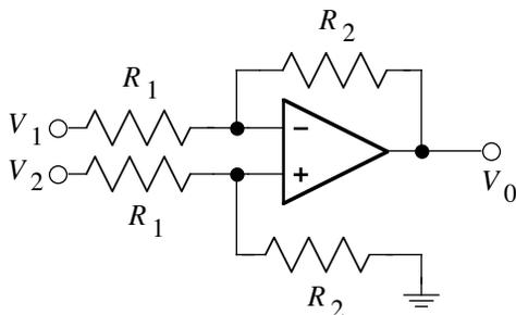
Infinite open-loop op-amp gain: virtual short rule:  $V_+ = V_-$
