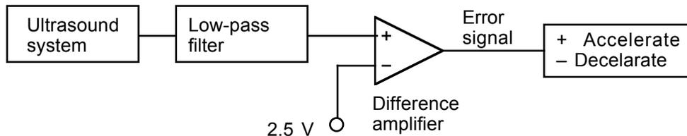
An alternative design uses a summing amplifier to take the difference between the average ultrasound ranging signal and the 2.5 V set point.
