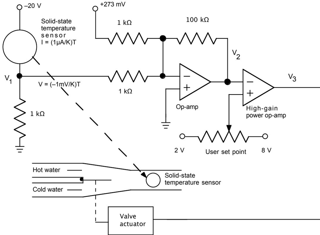
**5.2** The user set point is at 2.0V, and by the virtual short rule,  $V_2 = 2.0$  volts, which corresponds to a temperature of  $20^\circ\text{C}$ , as desired. The power op-amp output  $V_3 = -5\text{V}$ , as needed to pass only  $20^\circ\text{C}$  water through the mixing valve.
