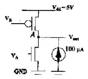
**1b**) (20 pts) Find the minimum value of (W/L)p such that when Va = 5V and Vb = 0V, the output voltage (including the 100 uA current) will be less than or equal to 1.5V. Note that both Va and Vb have changed from part a.
