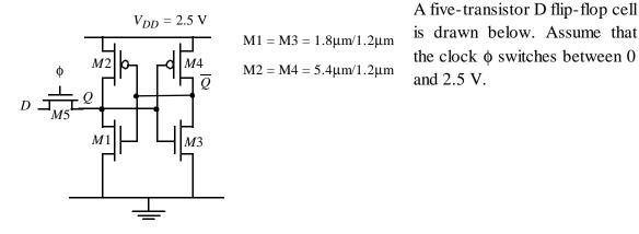
a. Determine the size constraints on transistor  $M_5$  so that a 0 can be written in the cell.
