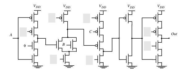
a. Fill in the missing clock connections on the schematics (marked by the gray boxes) so that the circuit will operate correctly. For each connection you can choose between  $\phi$  and  $\overline{\phi}$  (you may assume here that they are non-overlapping and that there is no skew).
