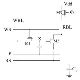
8(a) What are the voltages (Vdd or GND) required on the control signals (WS, RS) to read from this cell. (2 points)
