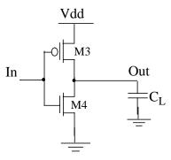
3(a) Vdd = 5V. What is the energy stored in  $C_L$  after it is fully charged? (2 points)
