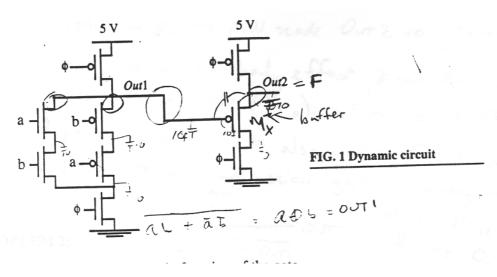
a. Determine the intended logic function of the gate.
