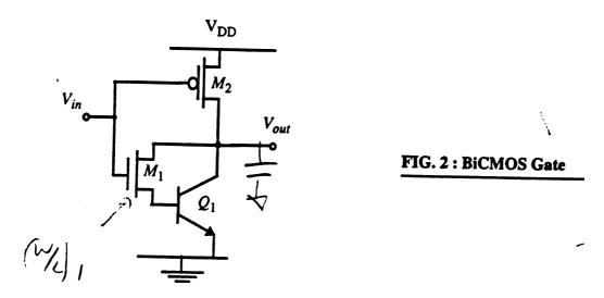
Determine the size of transistor  $M_2$  such that the gate displays similar values for  $t_{pLH}$  and  $t_{pLH}$ . You may assume that the load capacitance is huge and dominates the performance. The bipolar transistor is minimum size, while the size of  $M_1$  equals  $(W/L)_1$ . You may assume that the output swings from rail to rail. You may also assume that the MOS transistors stay in saturation during the transients. **Solve symbolically and do NOT fill in any numbers.**
