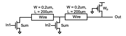
a) (6 pts) For the circuit shown above, size the PMOS pull-up transistor (i.e., choose W<sub>p</sub>) so that the pull-up resistance of the gate is equal to 4 times the worst-case pull-down resistance.
