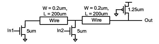
**b)** (10 pts) Assuming that you found that  $W_p = 1.25$ um in order for the pull-up resistance to be 4 times larger than the worst-case pull-down resistance (as shown above – note that this may or may not be the right answer to part a)), what is the worst-case ramp delay of the circuit?
