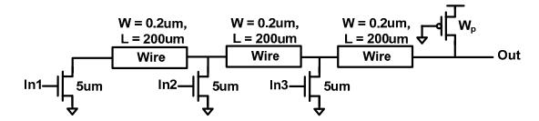
c) (6 pts) Assuming that every time you add another input to the circuit an additional 200um of wire is added as well (as shown above for 3 inputs), and that the pull-up transistor is always resized to make its resistance 4 times that of the worst-case pull-down resistance, what is the worst-case ramp delay of the circuit as a function of the number of inputs (N<sub>in</sub>)?
