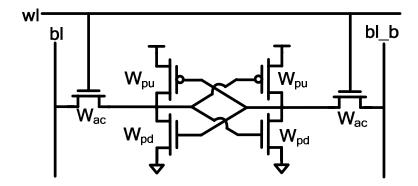
b) (8 pts) If we scale to a 50nm technology with fixed voltage scaling (i.e.,  $V_{DD}$  and  $V_{TH}$  fixed), recalculate the  $W_{pu}/W_{ac}$  required to maintain the same write margin as part a).
