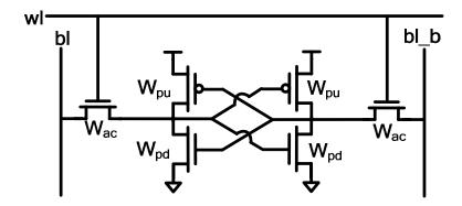
c) (4 pts) Given your answer to part b) and assuming that  $W_{pd}/W_{ac}$  is set to 1.5 independent of technology and that the area of the SRAM cell is set by  $W_{ac}*L+W_{pu}*L+W_{pd}*L$ , how many times reduction in area is achieved by scaling the SRAM cell from the 100nm technology to the 50nm technology?
