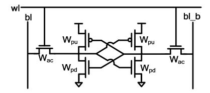
a) (6 pts) Assuming that the  $I_{DSAT}$  of the access transistor must be 1.5 times the  $I_{DSAT}$  of the pull-up transistor (i.e.,  $I_{DSAT\_ac} = 1.5*I_{DSAT\_pu}$ ) in order to ensure sufficient write margin, what should  $W_{pu}/W_{ac}$  be in our 100nm technology?
