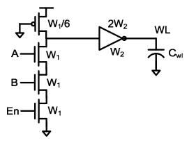
a) (6 pts) In units of  $t_{inv}$  and as a function of  $W_1$ ,  $W_2$ , and  $C_{wl}/C_G$ , what is the delay of the final decoder from A or B rising to WL rising?
