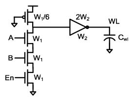
c) (6 pts) With f = 1GHz,  $W_1 = 2\mu m$ ,  $W_2 = 2\mu m$ , and  $C_{WL} = 50$  fF and as a function of  $V_{DD}$  and  $t_{inv}$ , what are the sensitivities  $S_{W1}$  and  $S_{W2}$ , where  $S_x = (\partial Power/\partial x)/(\partial Delay/\partial x)$ ?
