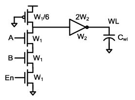
b) (11 pts) Assuming that the SRAM operates at a clock frequency of f, what is the average power consumed by this final decoder? You do not need to include the power consumed by driving the A, B, and En inputs, and you can assume that the En signal is a clock, but that it is only high 20% of the clock cycle. For simplicity you can also assume that the V<sub>OL</sub> of the ratioed gate is ~0V, and that the I<sub>DSAT</sub> of a PMOS transistor is equal to V<sub>DD</sub>/(R<sub>sqp</sub>\*L/W).
