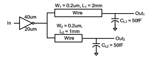
a) (8 pts) What is the ramp delay of the circuit shown above from In to Out<sub>1</sub>?
