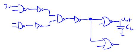
e) (8 pts) Now let's imagine that you are working in a new technology where the  $\gamma$  (= C<sub>D</sub>/C<sub>G</sub>) of the transistors is 100. Now how would you redesign the chain of gates in order to improve its delay? Please draw an improved schematic for the new chain of gates; you don't need to provide gate sizes. (You will receive partial credit if you can explain in general how  $\gamma$  should affect the design of the chain.)
