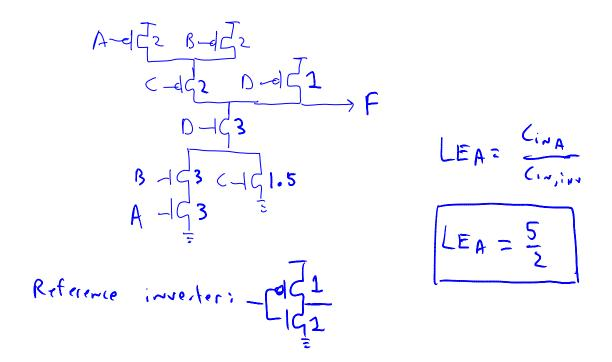
c) (12 pts) Using the switch model for the transistors, what is the worst-case delay of the gate shown below? You can assume that  $C_G = C_D = 2fF/\mu m$ ,  $R_{sqn} = 10k\Omega/\Box$ , and  $R_{sqp} = 20k\Omega/\Box$ , and you should provide your answer in ps.
