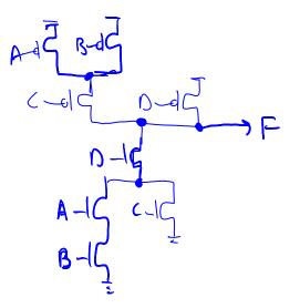
b) (4 pts) Assuming  $R_{sqp} = R_{sqn}$ , size your gate so that the worst-case pull up resistance is equal to the worst-case pull-down resistance. What is the logical effort of this gate from the A input?
