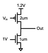
c) (6 points) How much total energy is dissipated by the inverter shown below when In steps from 1.2V to 0V and then back to 1.2V? You can ignore all capacitors associated with the transistors inside of the inverter.
