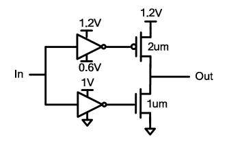
b) (6 pts) Using the velocity saturated model and assuming that both of the transistors below operate in saturation, what value of  $V_{in}$  makes the drain current of the two transistors equal to each other?..
