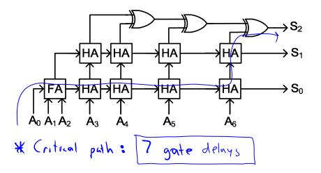
**b)** (4 pts) If each FA requires  $10\mu m^2$  of area, each HA requires  $6\mu m^2$ , and each XOR requires  $4\mu m^2$ , how much total area is occupied by the circuit from part a)?
