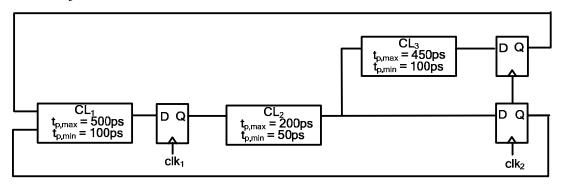
a) (6 pts) Assuming there is no skew between clk<sub>1</sub> and clk<sub>2</sub>, what is the minimum clock cycle time for this pipeline? Are there any minimum delay (hold time) violations?
