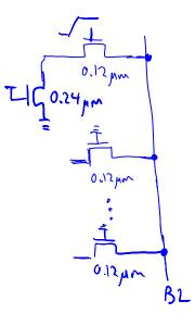
$$R_{cell} = LR_{syN} \cdot \left(\frac{1}{0.12\mu m} + \frac{1}{0.24\mu m}\right)$$
