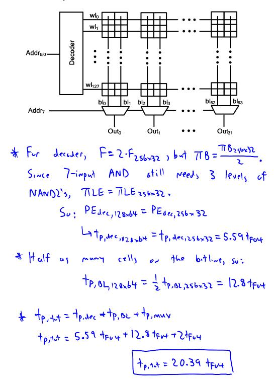
d) (8 pts) Now assuming that the SRAM is partitioned into a  $256/N_{part} \ge 32*N_{part}$  array, what value of  $N_{part}$  results in the minimum total delay for the SRAM? You should assume that the overall logical effort of the decoder is independent of  $N_{part}$ , and that the delay of an N-input MUX is N t<sub>FO4</sub>.
