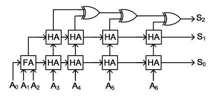
**b)** (4 pts) If each FA requires  $10\mu m^2$  of area, each HA requires  $6\mu m^2$ , and each XOR requires  $4\mu m^2$ , how much total area is occupied by the circuit from part a)?
