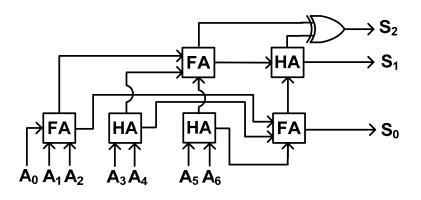
d) (10 pts) Still using only full adders, half adders, and XORs, and without increasing the delay, draw an implementation for this circuit that uses even less area than the one from part c). How much area does this implementation require?
