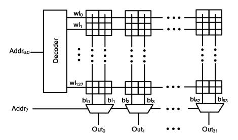
d) (8 pts) Now assuming that the SRAM is partitioned into a  $256/N_{part} \times 32*N_{part}$  array, what value of  $N_{part}$  results in the minimum total delay for the SRAM? You should assume that the overall logical effort of the decoder is independent of  $N_{part}$ , and that the delay of an N-input MUX is N t<sub>FO4</sub>.
