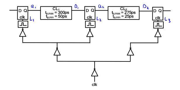
d) (10 pts) If we replace the flip flops by pulsed latches with the same  $t_{clk-q}$ ,  $t_{setup}$ , and  $t_{hold}$  as the flip-flops, and with  $t_{d-q} = t_{clk-q} + t_{setup}$ , can the minimum cycle time of the pipeline be reduced without potentially failing a minimum delay constraint? If so, how wide must the pulses be, and what is the new minimum cycle time? If not, explain which path fails the minimum delay constraint.
