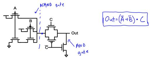
b) (7 pts) Given the sizing shown below, what value of W would you use in order to make the worst-case LE of the C input equal to half the LE of the A and B inputs (i.e.,  $LE_C = \frac{1}{2}LE_A$ )? What would be the LE of the C input in this case?
