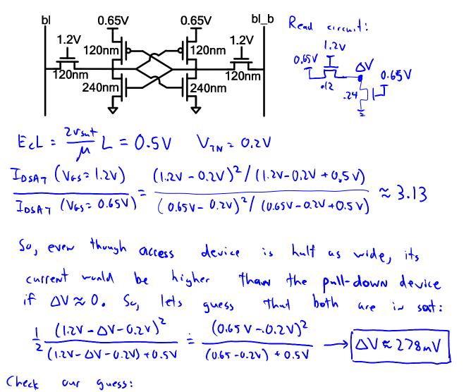
$$V_{0Taccess} = 1.2 V - 278 \text{mV} - 200 \text{mV}^{=} 722 \text{mV} \qquad V_{0SA77a} = \frac{722 \text{mV} \cdot 500 \text{mV}}{722 \text{mV} + 500 \text{mV}} \approx 295 \text{mV}$$
