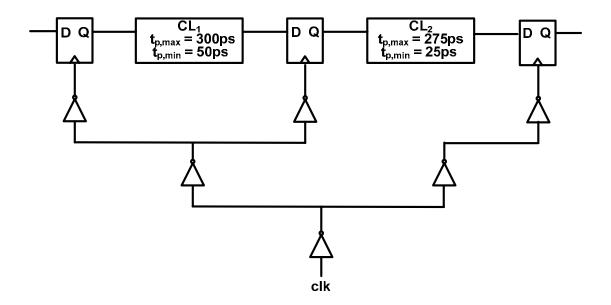
c) (4 pts) Under these same conditions (i.e., 50ps nominal inverter delay, +/-20% delay variation), can this pipeline fail any minimum delay constraints?
