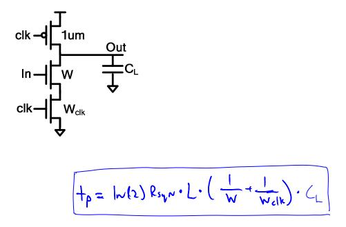
d) (2 pts) Assuming that In has an activity factor of  $\alpha_{0,1}$ , how much power is consumed due to driving In? How about due to driving clk? You should provide your answers in terms of W,  $W_{clk}$ ,  $\alpha_{0,1}$ , C<sub>G</sub>, V<sub>DD</sub>, and *f*.
