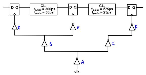
**b)** (4 pts) Now we'll include the clock distribution network for this pipeline. Assuming that the delay of each inverter is nominally 50ps, but that each inverter's delay varies randomly by +/-20%, now what is the minimum clock cycle time?
