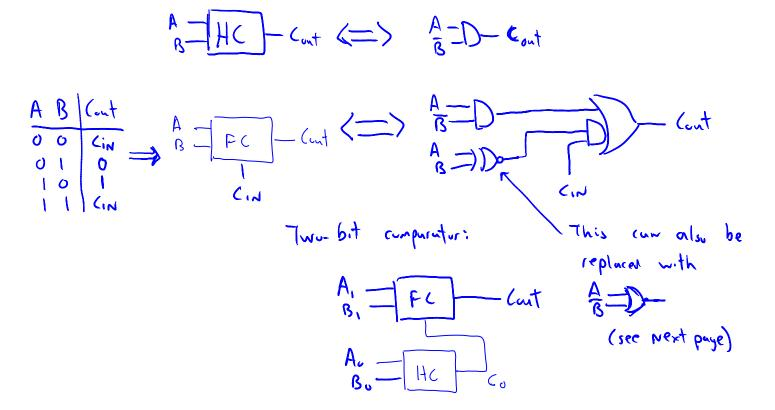
c) (5 pts) Notice that these comparators have several characteristics that are very similar to adders. As a function of A and B, define new P (propagate) and G (generate) signals that are appropriate for comparators, and then write the logic equation that gives the C<sub>out</sub> for a particular bit using P, G, and C<sub>in</sub>.
