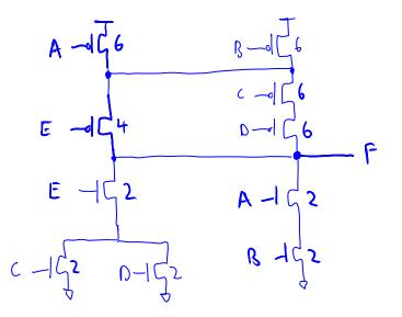
b) (3 pts) What is the logic function performed by the dynamic gate shown below?
