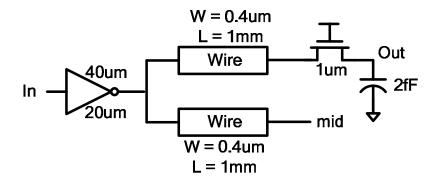
c) (12 pts) What is the ramp delay from In rising to Out falling for the circuit shown above? You do not need to provide a numerical answer for this problem – you only need to provide the equation you would use to calculate the delay, and the values of the R's and C's in that equation. You can assume that Out is initially charged to  $V_{DD}$ , and you can model each of the wires with a single section  $\Pi$  model.
