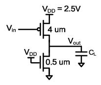
a) (6 pts) Using the unified transistor IV model, how much current flows from  $V_{DD}$  to Gnd when  $V_{in} = 0V$ ? (Hint: Think about the regions of operation – which transistor would have more current if both devices were velocity saturated?)
