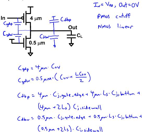
c) (4 pts) Now using the simplified capacitance model with  $C_G = 2 f F/\mu m$  and  $C_D = 1 f F/\mu m$ , how much dynamic power would a standard CMOS inverter with the same sizing (shown below) consume if In transitions from 0 to 1 every other clock cycle, the clock frequency is 100MHz, and  $C_L = 30 f F$ ? Don't forget to include the power consumption from driving the inverter's input capacitance.
