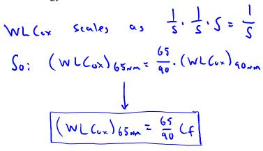
b) (5 pts) Given your answer to part a), how would the delay of an inverter with this C<sub>L</sub> scale from 90nm to 65nm?
