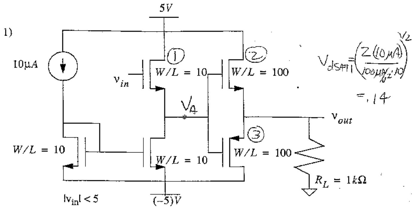
1. What is the maximum voltage at  $V_{out}$ ? 3.08V.
