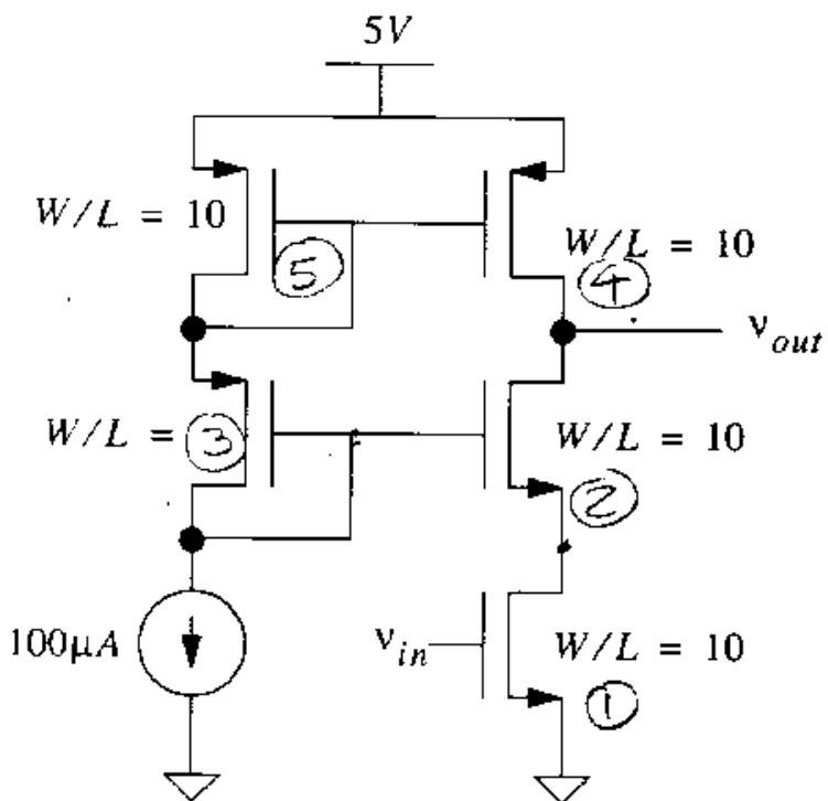
What is the value of the missing W/L so that the output swing is maximum?  $W/L = \underline{\underline{,43}}$
