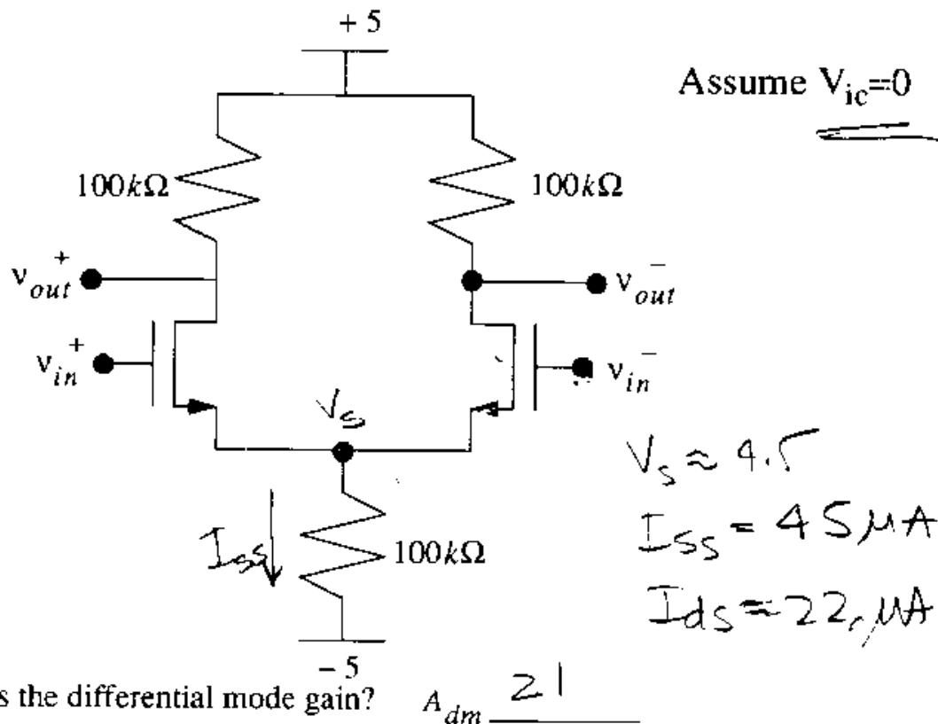
a) What is the differential mode gain?  $A_{dm} = \frac{21}{1 + 2g_m 100k\Omega}$
