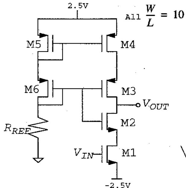
$$V_{dsAT} = \left( \frac{2I_D}{k'W/L} \right)^{1/2}$$
