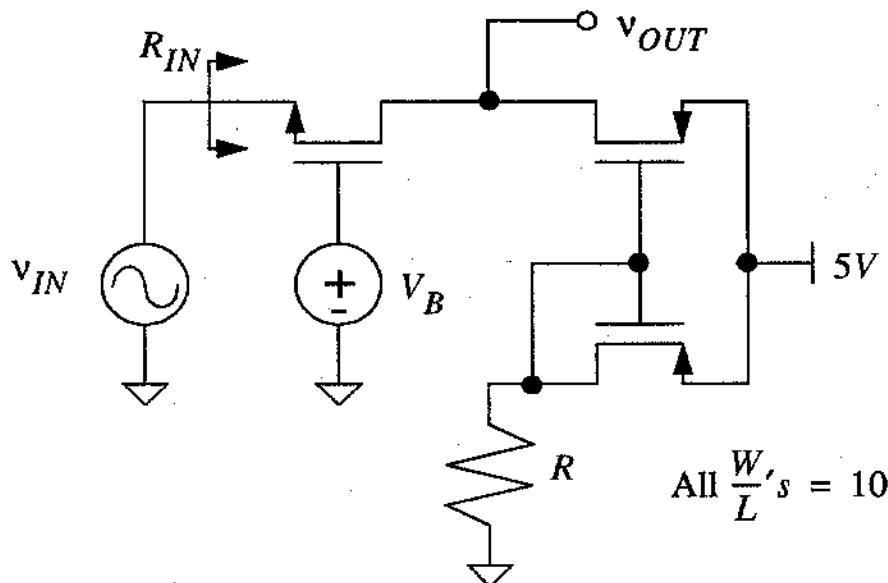
Assume  $R$  is chosen so that the currents are  $10 \mu\text{A}$  and  $V_B$  is chosen to set the DC voltage at  $v_{OUT} = 2.5 \text{ V}$
