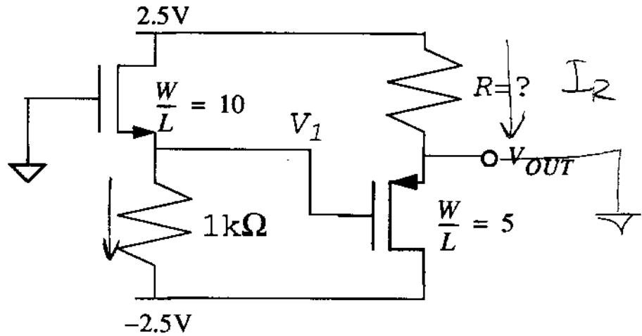
What is the voltage at  $V_1$ ? -1.74 V.
