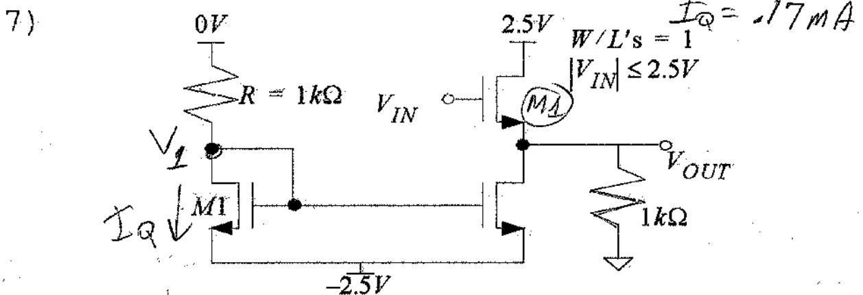
a) What is the most positive voltage that  $V_{OUT}$  can achieve? .027 Volts
