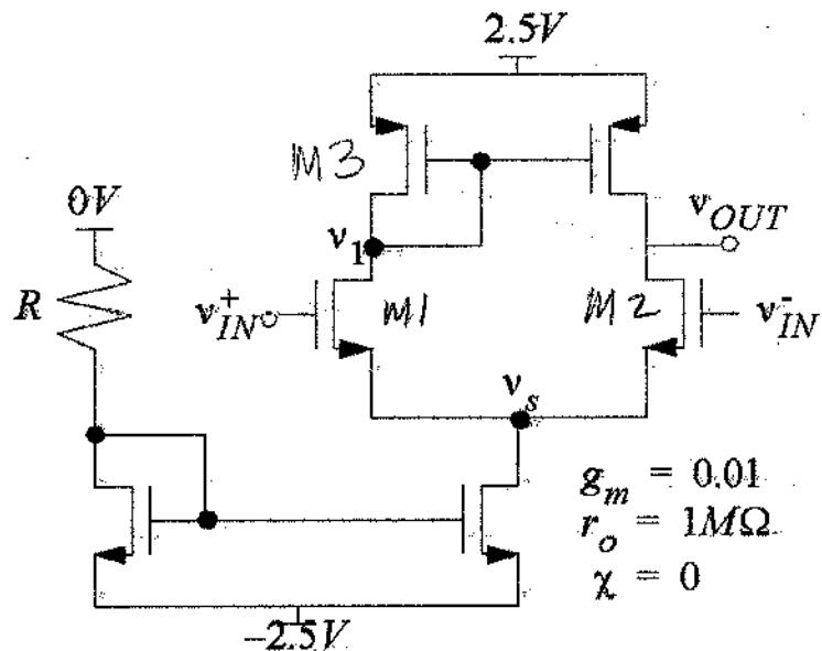
a) If  $v_{IN}^+ = v_{IN}^- = v_{IN}$ , what is  $v_s/v_{IN}$ ? 1
