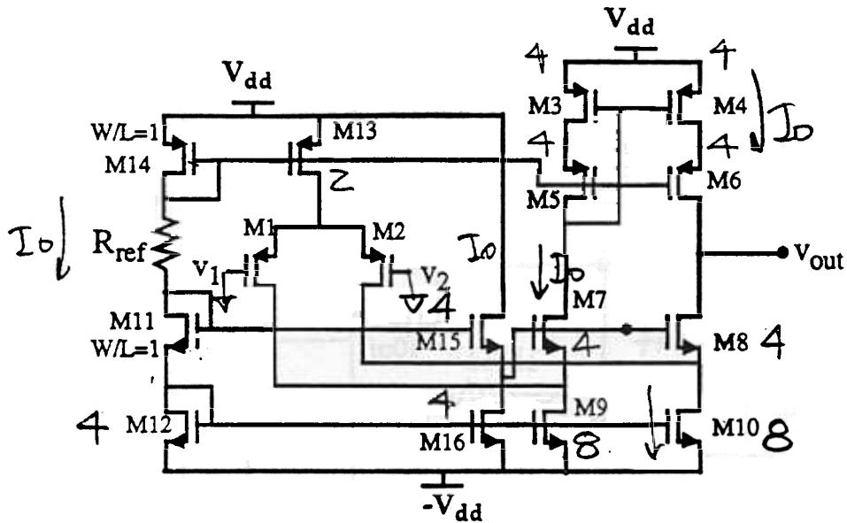
Choose the values of the W/L's for all the transistors (except for M11 and M14 which are 1), so that the currents in all transistors have the same value,  $I_o$ , except for M9, M10 and M13 which are twice that value or  $2I_o$ . Also, choose those sizes so that M3, M4, M9 and M10 are biased at the edge of saturation.  $\lambda=0$  for this problem.
