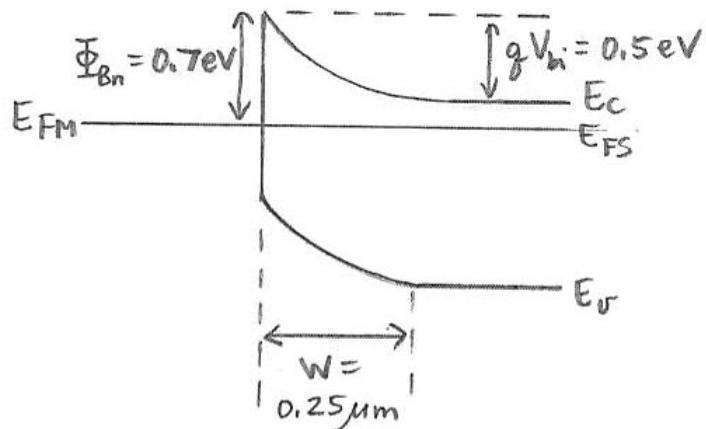
$$W = \sqrt{\frac{2\varepsilon_{Si}V_{bi}}{qN_D}} = \sqrt{\frac{2(10^{-12})(0.5)}{1.6 \times 10^{-19}(10^{16})}} = \sqrt{\frac{10^{-8}}{16}} = \frac{1}{4} \times 10^{-4} = \underline{0.25 \times 10^{-4} \text{ cm}}$$
