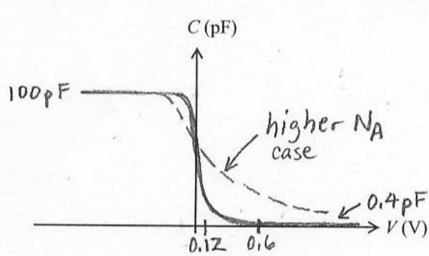
$$\frac{A}{C_{min}} = \frac{1}{C_{ox}} + \frac{1}{C_{dep}}$$
