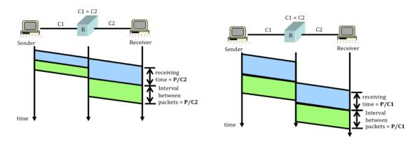
The above figure illustrates the impact of the relationship between link capacities in the case of a cutthrough router on (i) the inter-arrival between receiving the two packets, and (ii) the time it takes to receiving a packet. The packet length is P bits.
