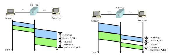
The above figure illustrates the impact of the relationship between link capacities on (i) the inter-arrival between receiving the two packets, and (ii) the time it takes to receiving a packet. The packet length is P bits.
