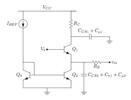
e) Find the input and output poles of this circuits. What is the dominant pole? Find the 3-dB bandwidth of this circuit. [5pts].
