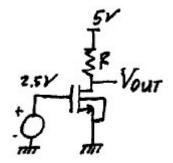
4.1 Find an expression for W so that the output voltage V<sub>out</sub> is 2.5V. Assume  $\lambda_n = 0.1 \text{ V}^{-1}$  when L = 1µm, and it is otherwise proportional to 1/L.
