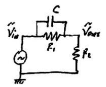
3.1 Write the transfer function  $v_{out} / v_{in}$ .
