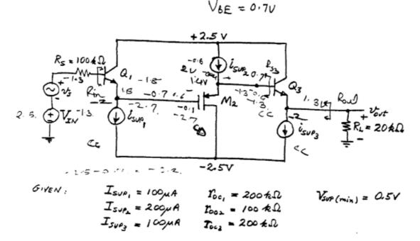
a) [4 pts.] What is width of transistor  $M_2$  such that the DC output voltage  $V_{out}=0$  V for  $V_{IN}=0$  V. Given: the length of  $M_2$  is  $L_2=2e-6$  m.
