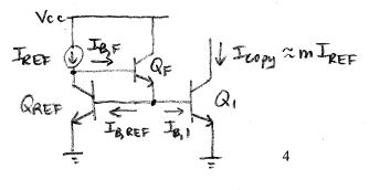
In this case, the fractional error is reduced by the factor B, since IBF = 1 (IB, REF + IB,1).
