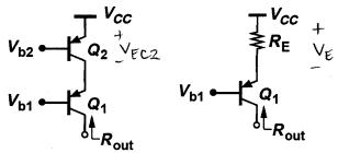
b) Suppose a PNP cascode is to be used as a 0.1mA current source, as shown below. What should be the values of the bias voltages  $V_{b1}$  and  $V_{b2}$ ? Assume that  $I_S = 10^{-16}$ A for each BJT, and that the  $Q_2$  collector junction is forward-biased by no more than 0.3V to ensure that  $Q_2$  operates in active mode.  $V_{CC} = 2.5V$ . Note that  $e^{0.72/0.026} \cong 10^{12}$ . [8 pts]
