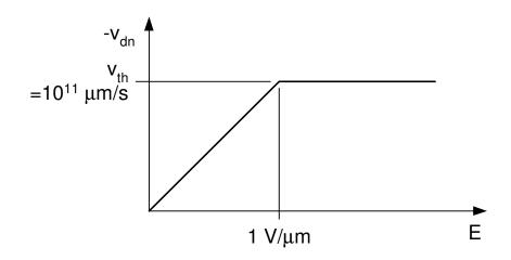
The above sketch shows a rough approximation of the electron drift velocity versus the electrical field in Silicon. For an NMOS transistor with L=0.1 $\mu$ m, W=10 $\mu$ m, and C<sub>ox</sub>=5fF/ $\mu$ m<sup>2</sup> calculate the following:
