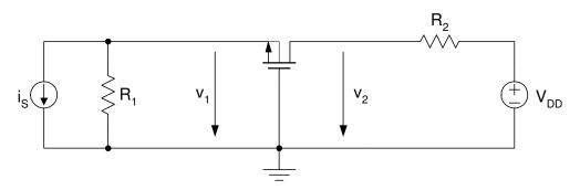
The circuit shown above is biased so that the transistor is in saturation.
