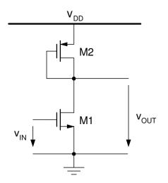
The circuit shown above is biased so that all transistors are in saturation. Draw a small signal model (label all elements with appropriate symbols, e.g.  $g_{m1}$ ,  $r_{o2}$ ) and find an *algebraic* expression for the small-signal voltage gain  $a_v = v_{out}/v_{in}$  as a function of small-signal parameters ( $g_m$ 's and  $r_o$ 's). Use  $g_m r_o >> 1$  to simplify your result.
