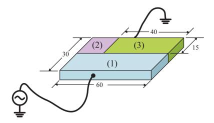
The sheet resistances of the region are  $R_{\Box}^1 = 10 \mathrm{k}\Omega/\mathrm{sq}, R_{\Box}^2 = 50 \mathrm{k}\Omega/\mathrm{sq}, R_{\Box}^3 = 30 \mathrm{k}\Omega/\mathrm{sq}.$
