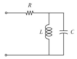
(a) Calculate the impedance transfer function. Identify the poles and zeros assuming that  $\omega_0 L/R = 10$ .
