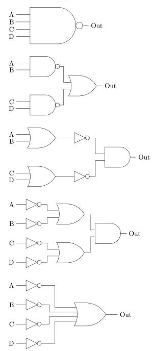
(b) 2-input NOR gates are said to be complete because any Boolean function can be computed with them. Prove this fact. Hint: implement a subset of the standard gates (AND, NOT, OR, NOR, NAND, XOR, XNOR) using just NOR gates, then apply a standard boolean algebra technique using these gates.
