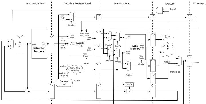
a. Assume that this pipeline resolves control hazards by pipeline stalls. How many cycles is it stalled on a control hazard?
