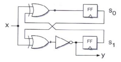
(b) In the diagram below, finish drawing in the *state transition diagram* for the circuit shown on the previous page (reproduced above). The bubbles below represent the possible states of the circuit as represented by the values held in the flip-flops, s1s0.
