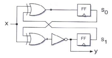
The xor gate and the inverter each have a propagation delay of 1ns. Flip-flops are *positive* edge-triggered and have a set-up time and clock-to-q delay of 1ns each.
