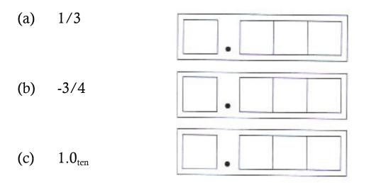
Suppose we have an 8-bit floating point number representation based on the principles of the IEEE 754, with the sign-bit (8), exponent (E), and the mantissa (M) fields as shown below. (You will need to adjust the exponent "bias" accordingly.)
